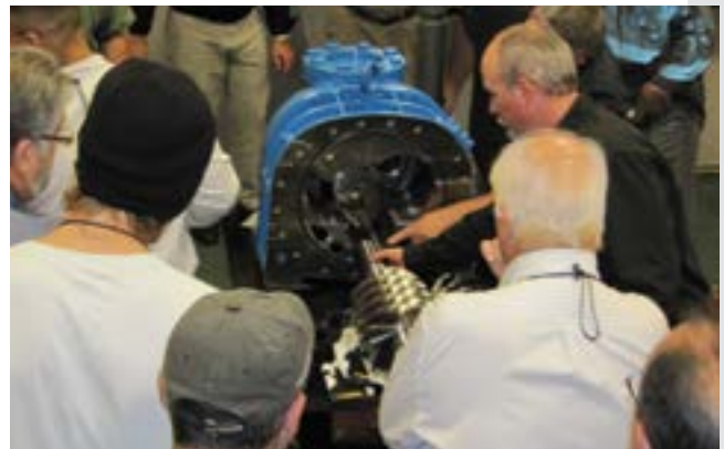
As an industry leader, GEA is privileged to educate and share technical knowledge with fellow industrial refrigeration professionals. Here, a GEA compressor rebuild specialist performs a screw compressor teardown for attendees of a Refrigerating Engineers & Technicians Association (RETA) annual conference.
