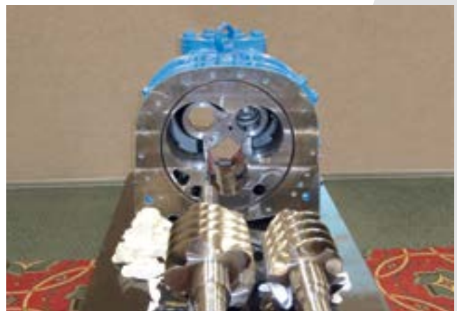
As an industry leader, GEA is privileged to educate and share technical knowledge with fellow industrial refrigeration professionals. Here, a GEA compressor rebuild specialist performs a screw compressor teardown for attendees of a Refrigerating Engineers & Technicians Association (RETA) annual conference.
